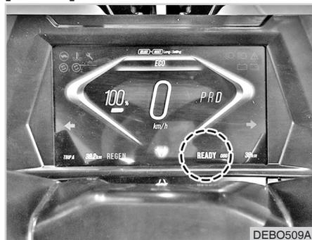
9. While holding the rear brake lever, press and hold the Ready button on the right-hand handle for 2 seconds, and verify that the READY indicator on the instrument panel illuminates.
