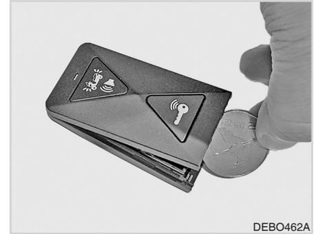
1. Remove the insert key (physical key) from the smart key body.
