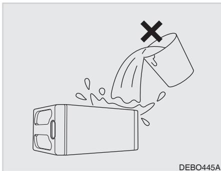
Avoid dropping the battery into water. If dropped carelessly, it may not function properly.
