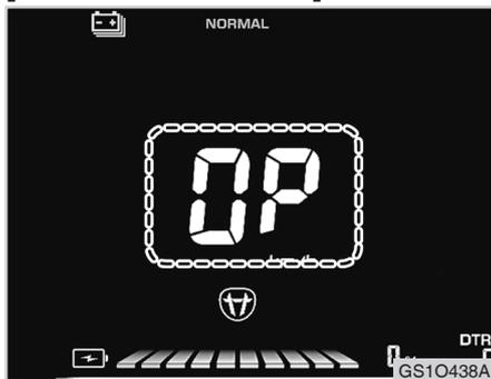
When the battery cover or seat is opened, the digital speedometer display shows "OP."
