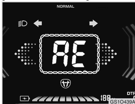
When reversing, the digital speedometer display shows "RE" and the turn signal lamps (hazard warning lamps) are activated simultaneously.
